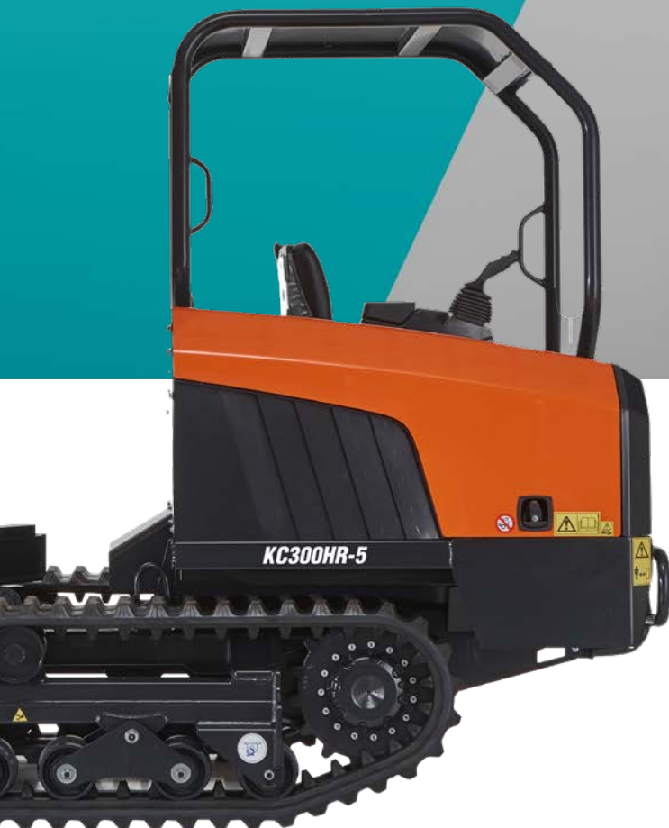
KC300HR-5 (180° rotary dumping function)
